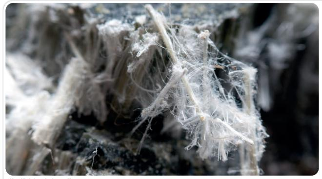
Magnified view of asbestos fibre
